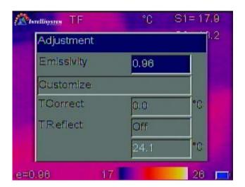
Press **Menu** key to activate the main menu. Select **Setup->Adjustment** and press **Confirm** key to pop up the Adjustment dialog box. User may set emissivity, temperature correct and ambient temperature. Press **Up** and **Down** keys to choose different items, **Left** and **Right** keys to modify the item contents.
