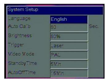
Press **Menu** key to activate the main menu. Select **Setup->Sys. Setup** and press **Confirm** key to open the **System Setup** dialog box. User can set Language, Auto calibration, LCD brightness, Trigger assignment, Video mode, Standby time and Auto off time. Press **Up** and **Down** keys to choose menu items, **Left** and **Right** keys to modify the item contents.
