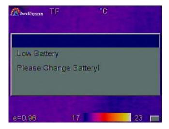
When battery has approximately 5% charge remaining, the warning will be displayed and the instrument will turn off in approximately 3 seconds.
