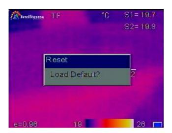
It is used for resetting factory defaults. Press **Menu** key to activate the main menu. Select **Setup->Default** and press **Confirm** key to open the **Reset** dialog box. Press **Confirm** key to reset the factory default. Press **C** key to cancel the reset operation. Appendix B indicates the detailed factory default parameter table.
