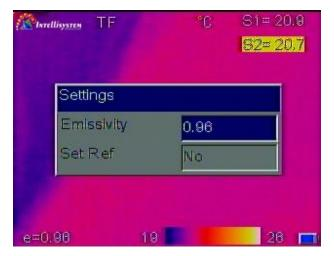
Spot settings include emissivity and reference temperature. When Set Ref
