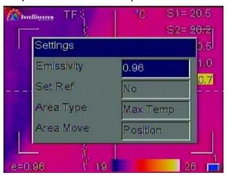
Area settings can modify the emissivity, area measurement type and area move parameter. Measurement types are Min Temp, Max Temp or Average Temp. Area Move parameter choices are Position or Size. The selected parameter will be adjusted by the directional arrow keys. When "Set Ref" is set as **Yes**, the displayed values of other measurements will be their delta from this measurement.
