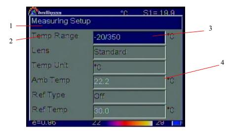
[1] **Dialog box name:** Displays the dialog box name, e.g. Measuring Setup.
